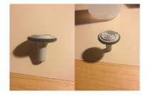
• Attach block into center of metal circle block below. Using tall, black handle on left, screw block into place. The center, black handle should also be tightened before cutting sections. Loosening this handle allows you to change the angle of the block face.
